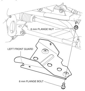
2. Loosely install the front guard brackets as shown.
